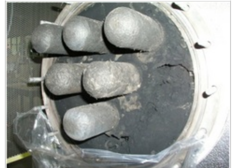
Ceramic candle filter for hot ash cleaning of raw woodgas, after 400 h of operation (480 kg wood).
