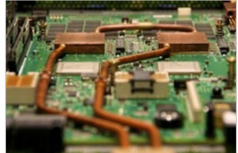
Liquid-cooling circuits on a prototype blade.
