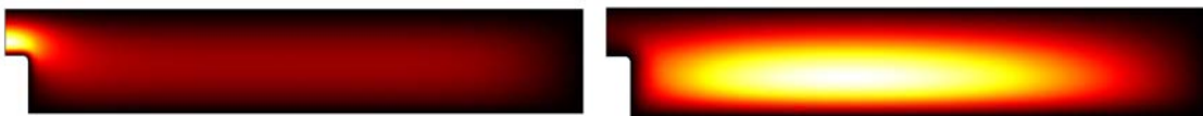
Figure 6: Numerical Simulation of electron density at a pressure of 5 mbar (left) and 0.8 mbar (right)
