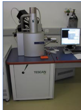
Below: The indenter stage from Hysitron, which was adapted for a SEM (left) and The Orsay Physics ion gun integrated into a Tescan SEM (right) at the Empa Thun.
