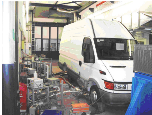
Fig. II-1: Vehicle for Diesel Oxidation Catalyst (DOC) application on the chassis dynamometer with the specifically designed exhaust aftertreatment housing (recognisable behind the right front wheel of the vehicle)
