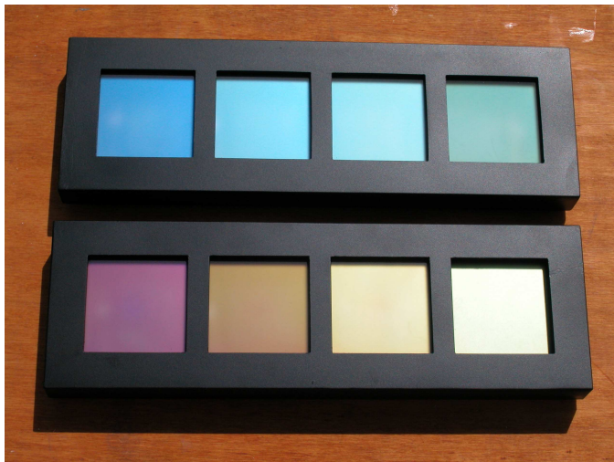
Figure 3: Mini demoboxes with coloured collector glass samples
