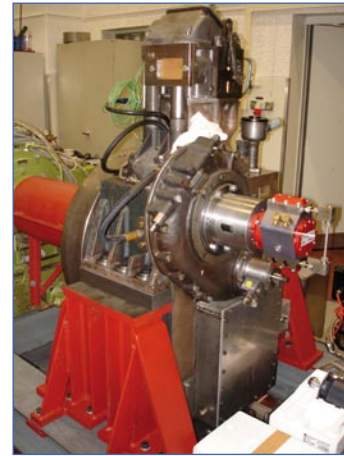
Single Cylinder Research Engine test facility as it is currently under construction.
