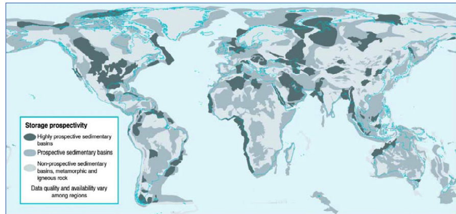
Figure 3: Prospective areas in sedimentary basins where suitable saline formations, oil or gas fields, or coal beds may be found (IPCC, 2005).
